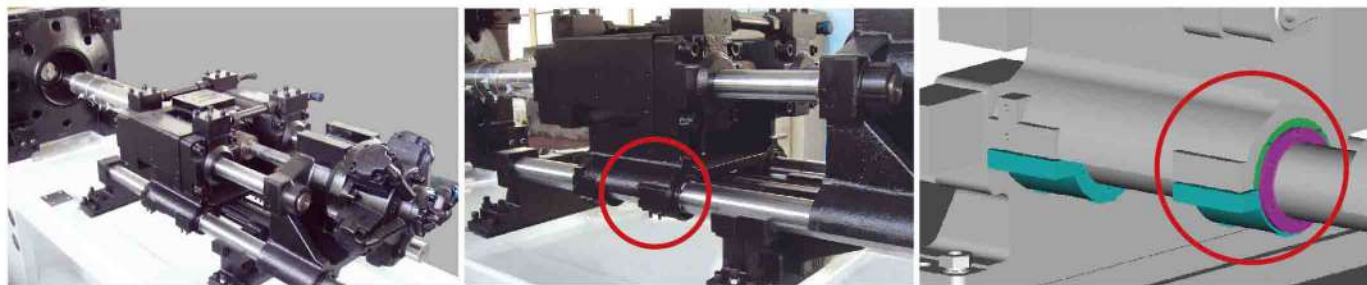
The injection assembly is guided with patented molybdenum disulfide coated bearings.
