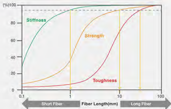
Figure 1 Diagram for the relationship between fiber length and stiffness, strength and toughness
