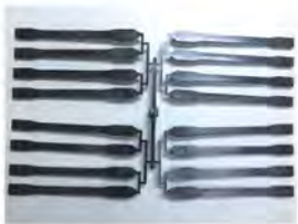
Figure 4 Physical diagram of tensile specimen Machine test and result
